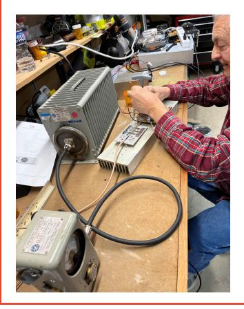
We drilled and tapped holes in the heat sink that aligned with the holes in the copper pallet and mounted the pallet along with a W6PQL low pass filter.
